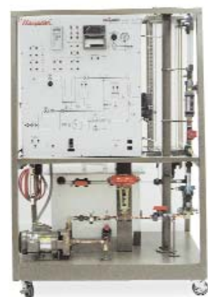
MODEL H-ICS-LT Level Process Control Trainer
