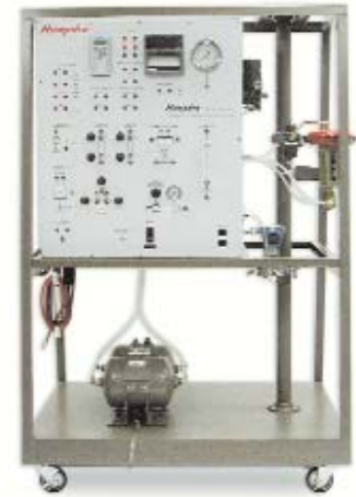
MODEL H-ICS-PT Pressure Process Trainer
