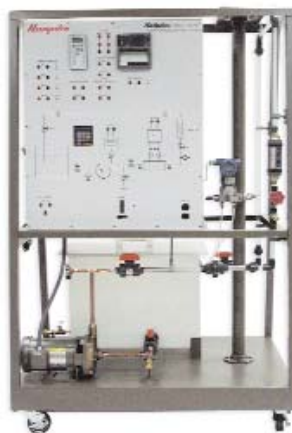
MODEL H-ICS-FT Flow Process Control Trainer
