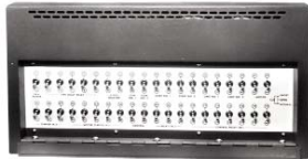
◀ Shorted and open components and circuits are simulated with fault switches on rear of unit.
